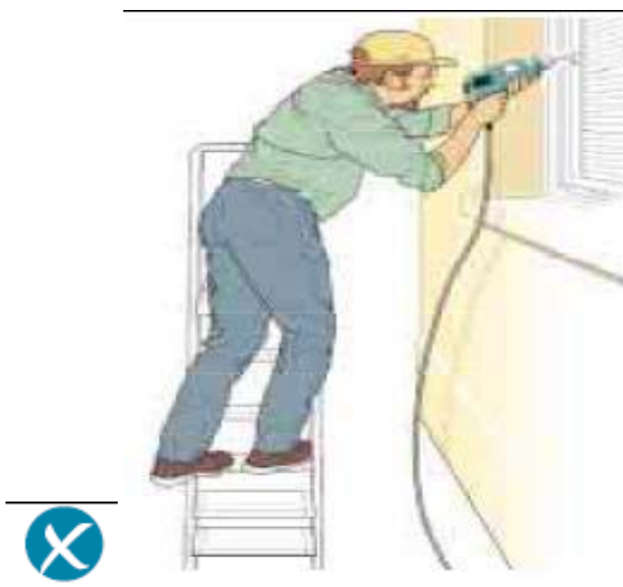
Incorrect – steps side on to work activity
